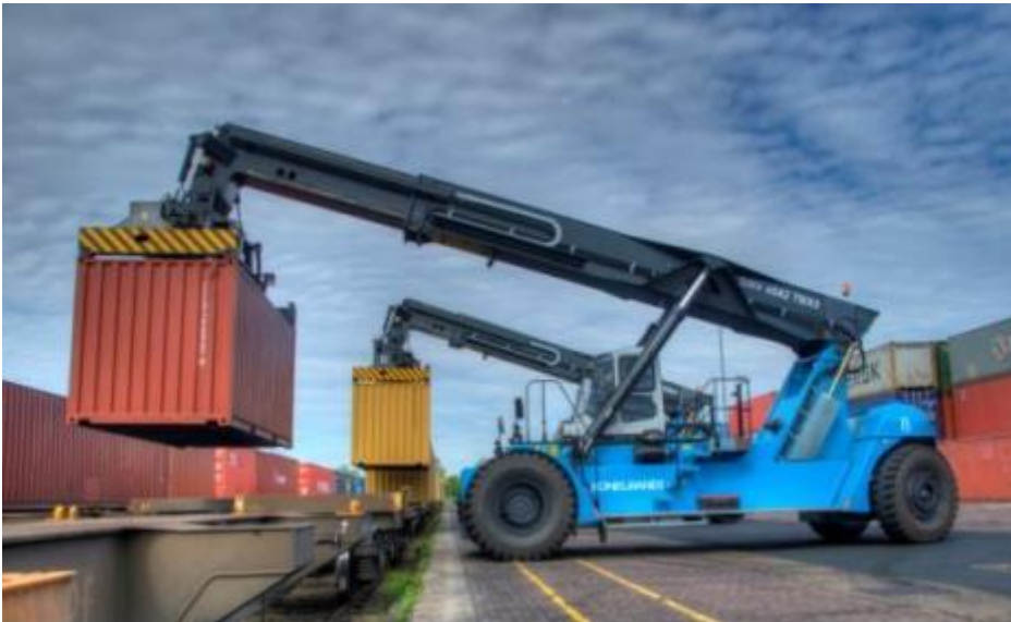
Figure 4.2- Example Reachstacker Operation – Hams Hall Rail Freight Terminal
