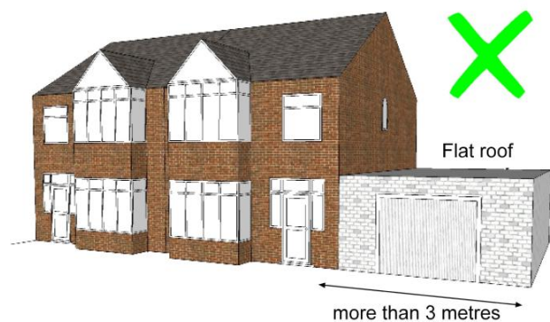
Figure D.2 Unbalanced prominent side extension
