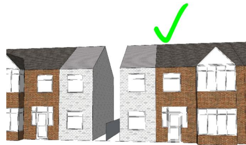
Figure E.1 Non-terracing side extension
