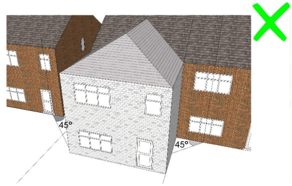
Figure C.4 Extension encroaches into 45 degree rule
