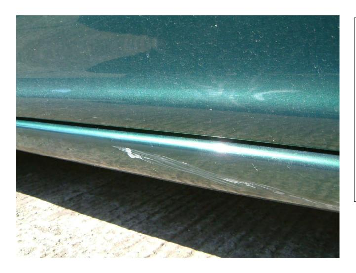
Excessive scratches or abrasions are unacceptable.
