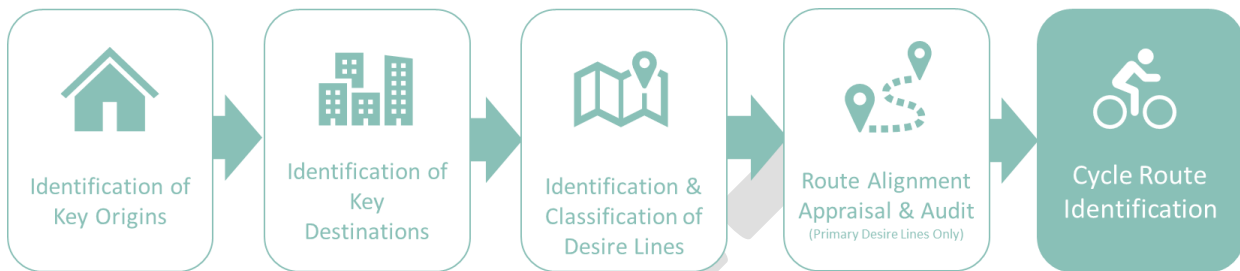
Figure 5-1: Cycling Network Development Process
